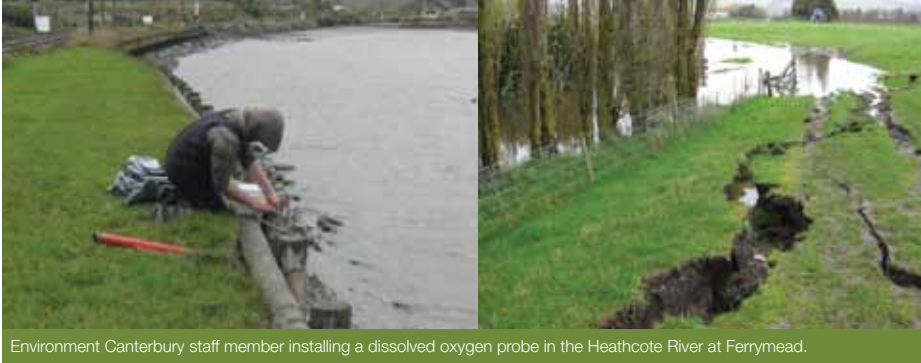
Environment Canterbury staff member installing a dissolved oxygen probe in the Heathcote River at Ferrymead.
