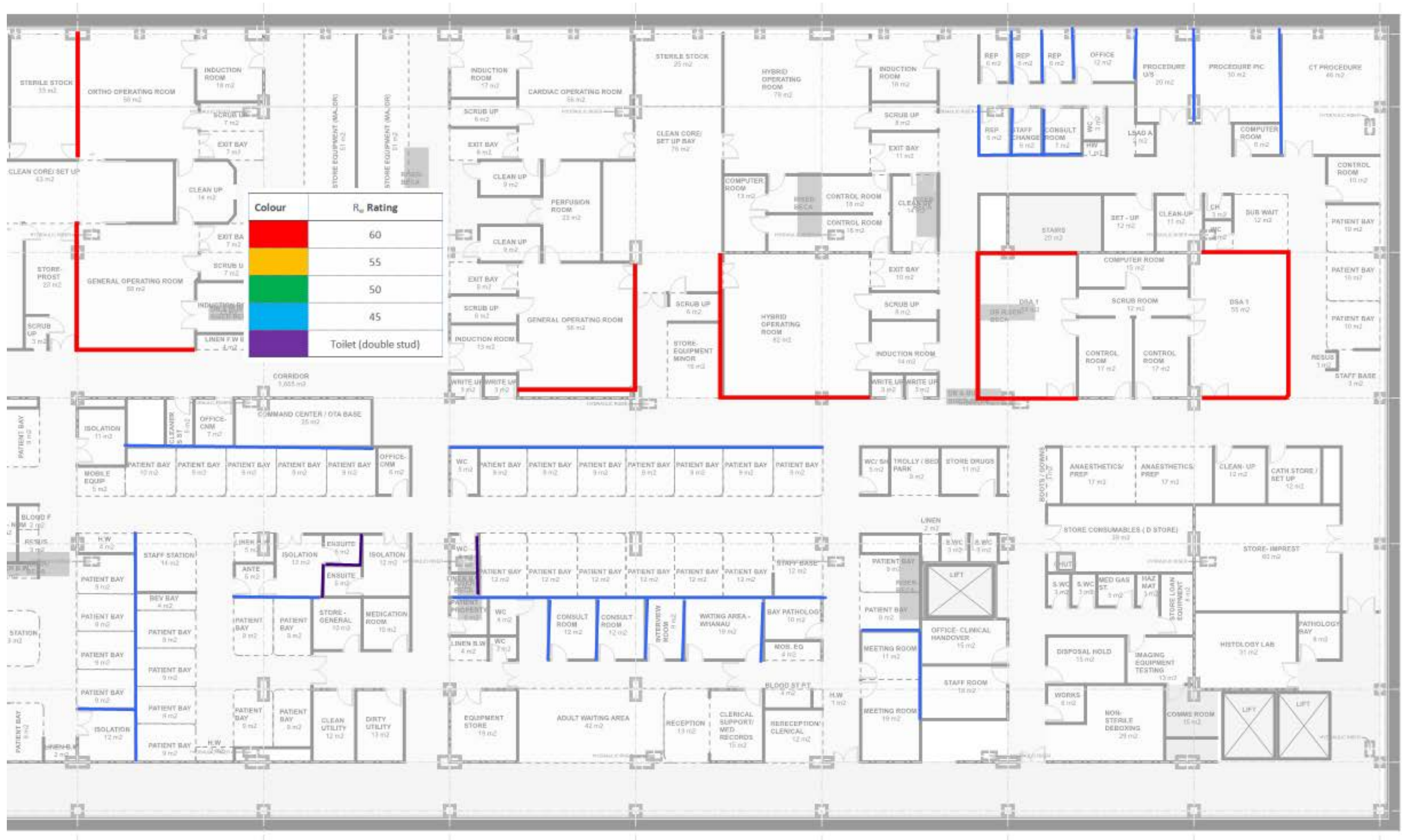
Figure 4: Typical Operating Theatre Partition Types
