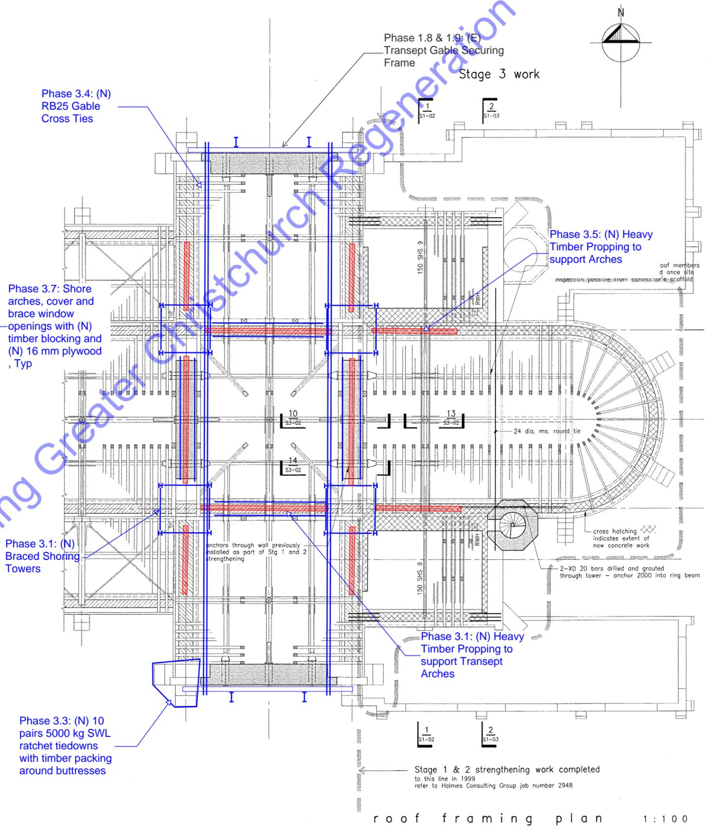
**STABILISATION - PHASE 3 GROUND FLOOR & ROOF PLAN**
