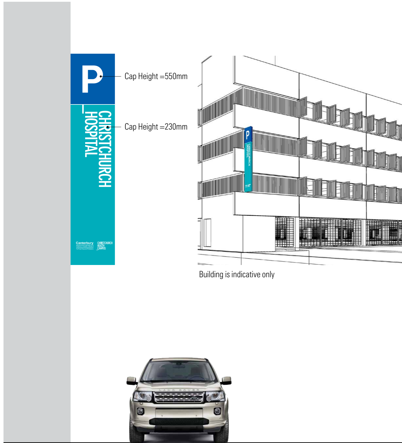
Car Park Building Identification - Perpendicular to traffic & building facade 900x4000 nominated subject to architecture Code EX-CBI
