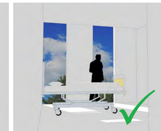
STUDY 04: 50% glazing with full height glazing on a 1m module. The views created by making the glazing full height feel generous and offer views down the park.
