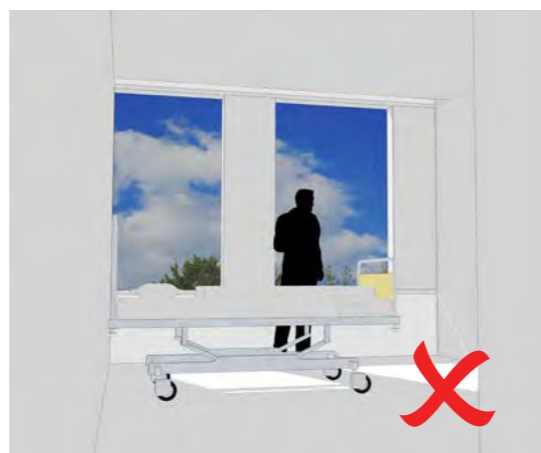
STUDY 01: 50% glazing with 800mm upstand. Having an upstand blocks views down to the park from the bed and lacks any unique character.
