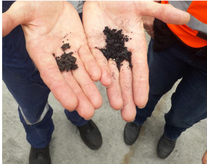
Biosolids from wastewater treatment following drying (left) and gasification (right).
